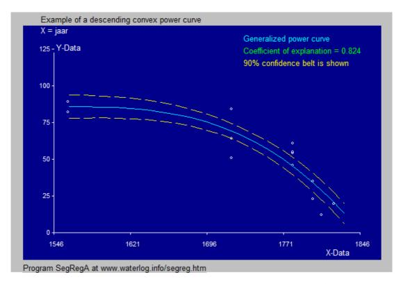
Figure D. Convex descending power curve  $Y = -0.0000032 (X-1554)^{3.0} + 85.9$
