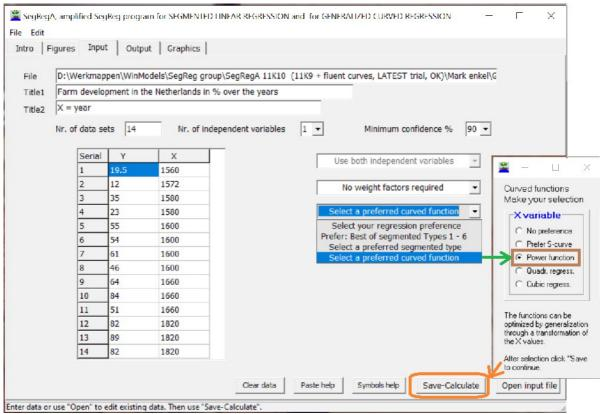
**Figure 3**. Input user interface of SegRegA. The input data are entered in the table. The selection box has been set to "Select a preferred curved function, blue rectangle), whereafter the option "Power function" has been selected (brown rectangle). The calculator gives the possibility to use more than 1 independent variable as well as the determination of the confidence level (here 90%). The calculations are done clicking the "Save-Calculate" button (orange rectangle).
